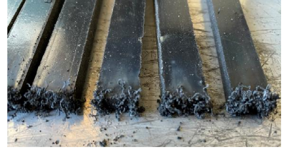
The EPDM-intumescent filler testpieces after testing
