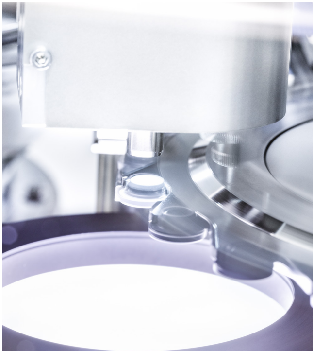
The FirstLine® concept includes high-level camera inspection to detect and remove defects before Datwyler's products are packed and shipped to its customers.
